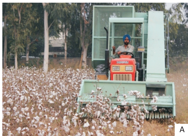
Figure 1. Operational view of tractor operated cotton stripper (A) and cotton picker (B)
