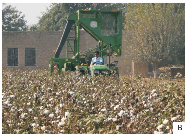
Figure 1. Operational view of tractor operated cotton stripper (A) and cotton picker (B)
